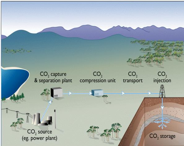
*In CCS, CO<sub>2</sub> is captured before it can be emitted into the atmosphere. It is then compressed into a dense fluid, transported to the injection site and disposed of underground in suitable rock formations.*
