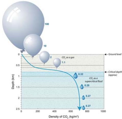
*CO<sub>2</sub> will be injected at depths below 0.8 km (2600 feet). CO<sub>2</sub> increases in density with depth and becomes a supercritical fluid below 0.8 km. Supercritical fluids take up less space and diffuse better than either gases or ordinary liquids through storage rocks. The blue numbers show the volume of CO<sub>2</sub> at each depth compared to the volume of 100 at the surface.*
