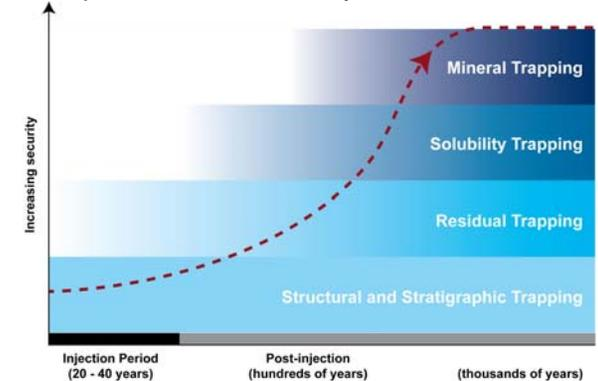
*As time goes on, increasingly secure trapping mechanisms come into play and the overall security of storage increases.*
